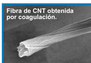
CNT fibre obtained by coagulation spinning
